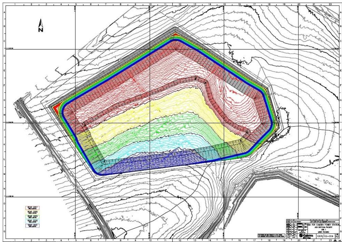
**Figure 6-3: Lining requirements for the first five (5) years of ash disposal**
