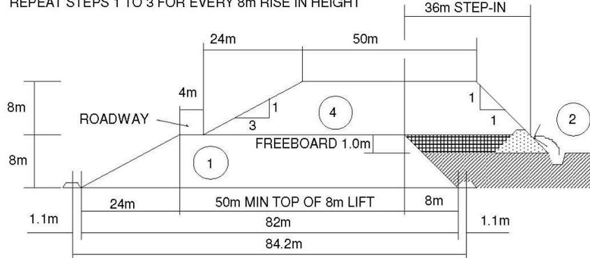
**Figure 7-4: Day wall step-in process**
