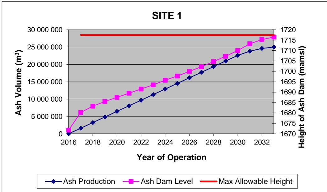
Figure 6-6: ADF Stage Curve for Site 1
