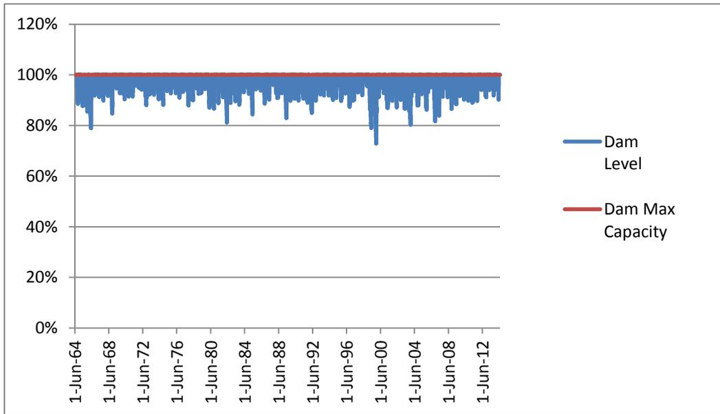
**Figure 5-3: Proposed New AWRD Levels for Simulation Period**
