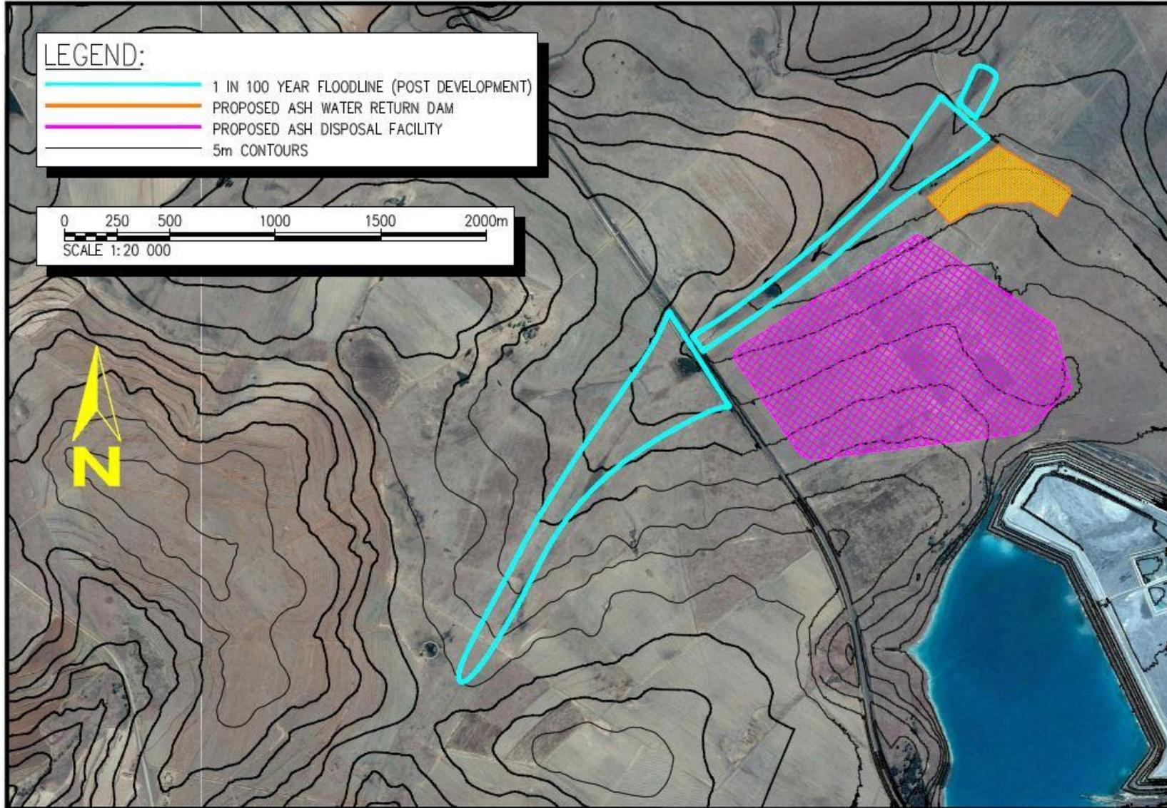
Figure 6-5: Resulting Post-Development 1 in 100 year Floodlines
