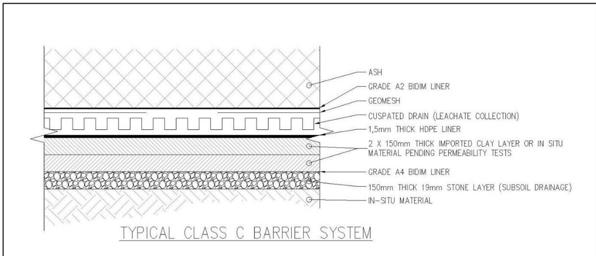
**Figure 6-1: Class C Landfill Barrier System**
