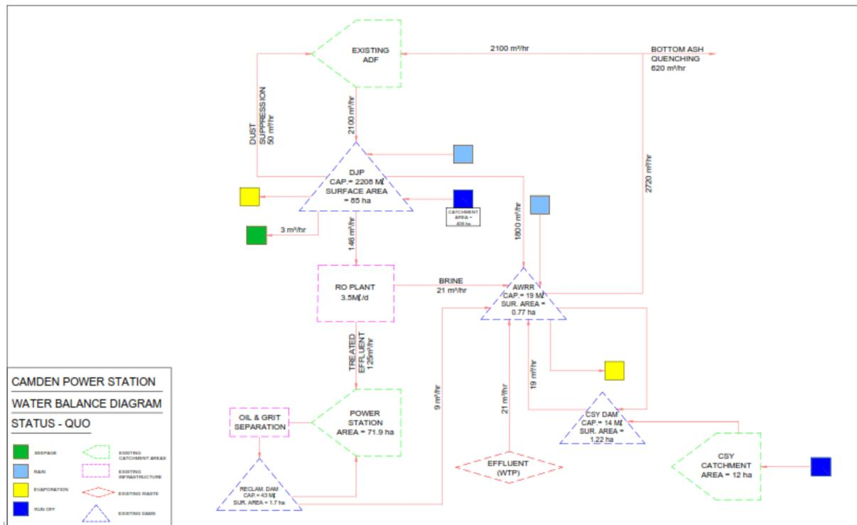
**Figure 5-1: Stormwater System Diagram – Status Quo**
