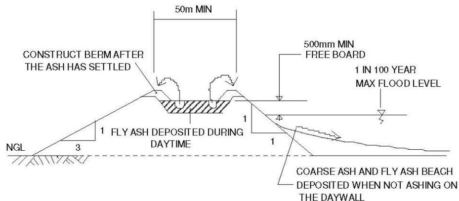
**Figure 7-3: Wall building method**
