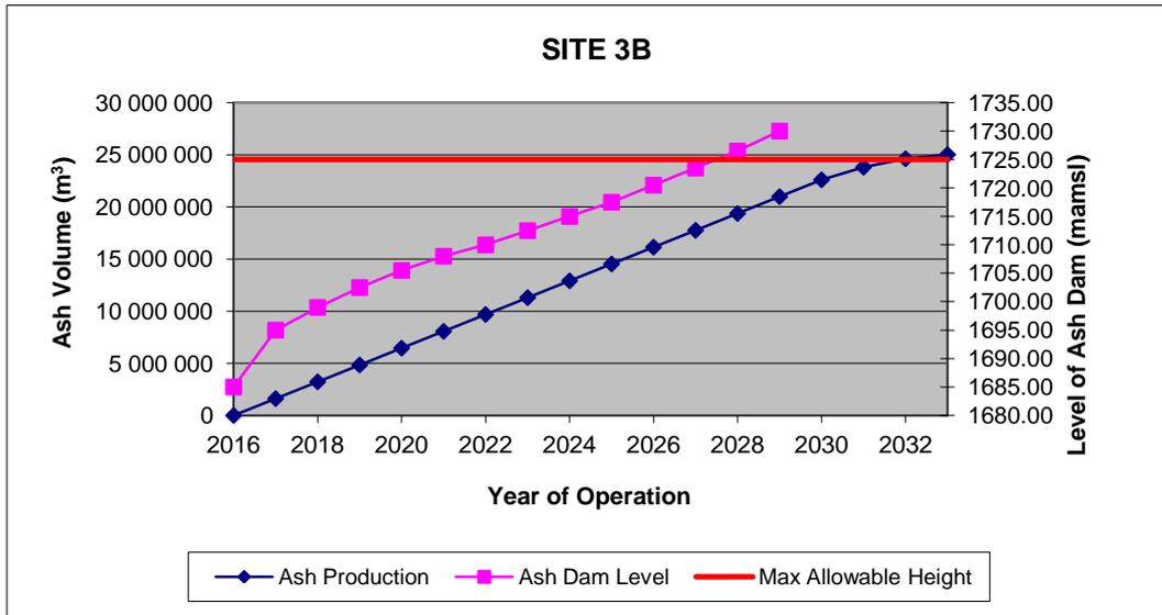
**Figure 6-8: ADF Stage Curve for Site 3B**
