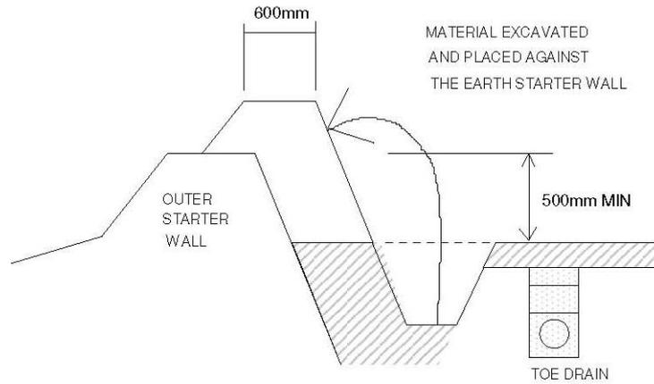
**Figure 7-2: Construction of first berm and step**
