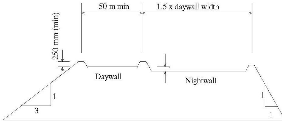
**Figure 7-6: Day wall and nightfall construction**
