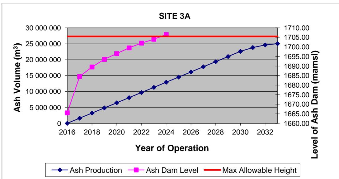
Figure 6-7: ADF Stage Curve for Site 3A
